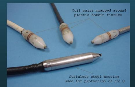
Outside Diameter (O.D.) probes are coils that are wound the circumference of a hollow fixture. The coil is designed such that the test part is ran through the middle of the coil. These probes can be used to inspect bars, rods as well as tubes.
