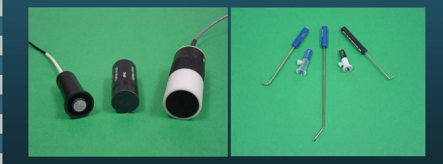
Some surface probes are specifically designed for crack detection of fastener holes. These include sliding probes, ring probes and hole probes.
